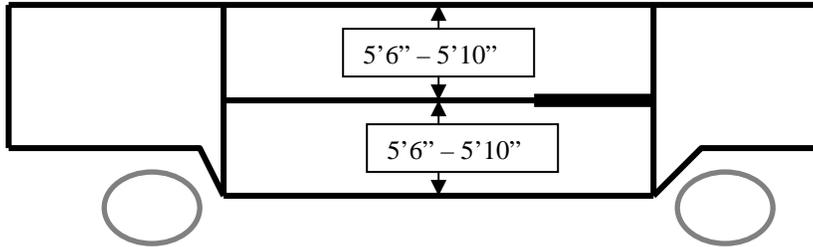
The lower deck also has a ramp stored, affixed to the lower deck ceiling, further reducing head-space by several inches for that area.
